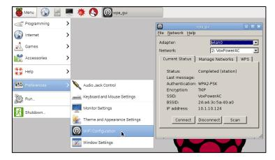
2 Click on the scan button and a second window will open. This new window lists all of the wireless network access points that the Pi can currently detect. Find yours and double click on it.
