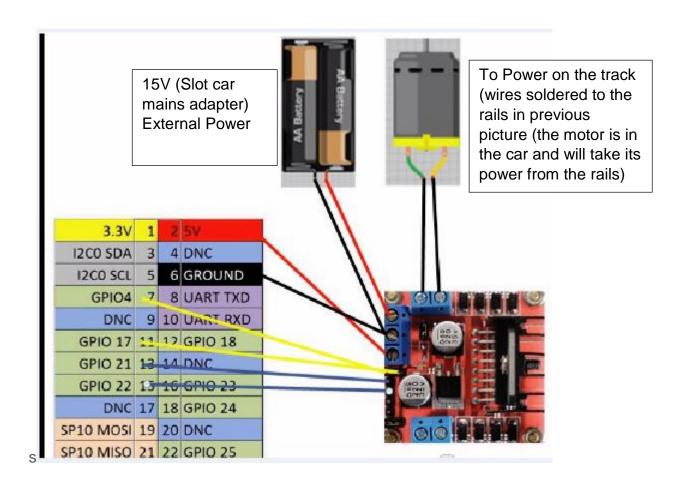
You will need to common the GND between the controller and the Pi hence the BLACK wire connected to pin 6.
