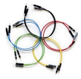
For making connections within your breadboard (to a different physical area) and to the Arduino itself, jumper wires are used. These are just bits of wire with fixed ends that can be stuck into the Arduino and plugs on the breadboard.
